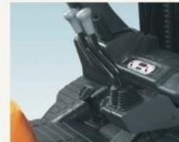
Multi-cone synchronizer shift levers The newly adopted levers enable smooth shifting from both forward and reverse (available for manual transmission models).
