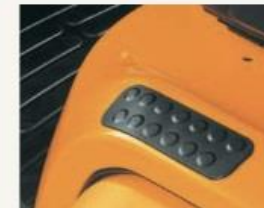
Anti-slip mat on the hood A rubber strip is attached to the hood to prevent slippage while stepping on and off.
