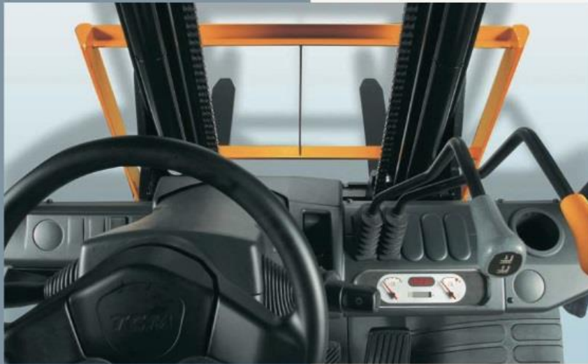
Reduced fatigue due to a semi-circular steering wheel A smaller diameter (300mm outer diameter) steering wheel gives improved vehicle maneuverability. In addition, this compact steering wheel makes it much easier to get on and off the truck.
