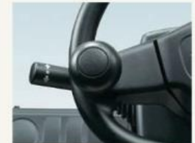
Neutral safety mechanism This feature enhances safety of operation. The engine cannot be started unless the change lever is in the neutral position.
